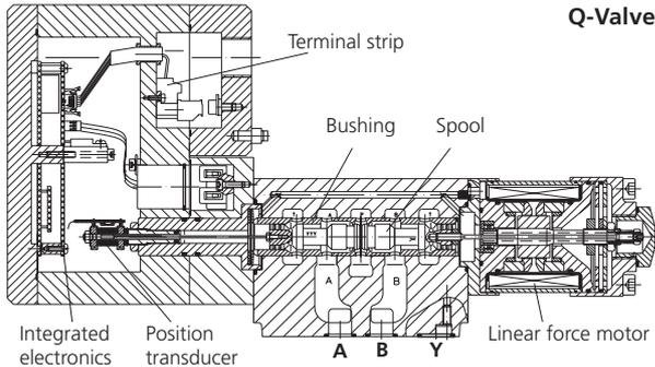
drive is a permanent magnet linear force motor which actively strokes the spool from its spring centred position in both directions. The closed loop spool position electronics and pulse width modulated (PWM) drive electronics are integrated into the valve. This permits control of the valve directly from, for example, a machine control without the use of additional interface electronics.
