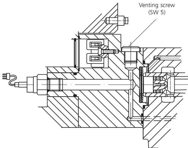
With pressure command set and lowered supply pressure, carefully open the venting screw by turning it **approximately one turn**. The entrapped air should escape now together with hydraulic fluid. Wait until no more air bubbles can be seen in the oil. Then close the venting screw and torque it to **10 Nm**.
